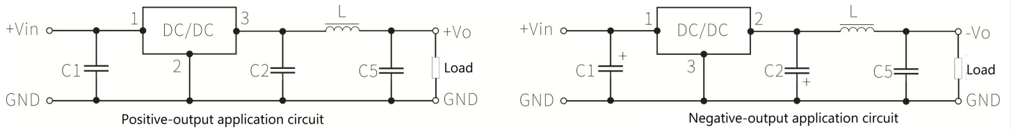
Figure 3: "LC" Filter Application Circuit
